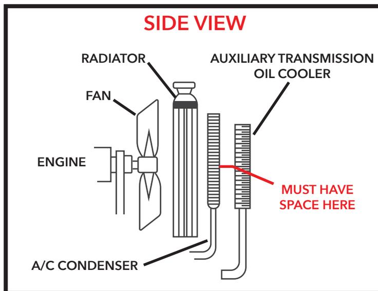
2. Find the two steel tubes (transmission cooler lines) running from the transmission to the original equipment cooler/radiator.
