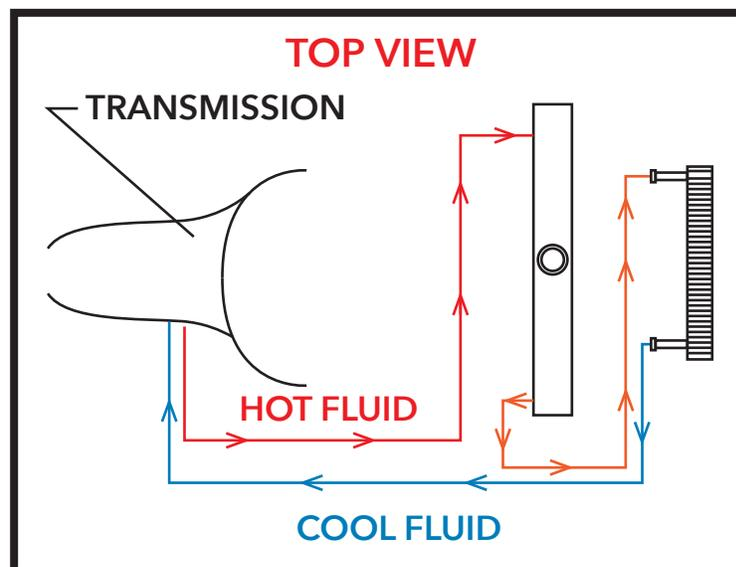
1. Hot transmission fluid flows from the transmission to the engine's radiator.
