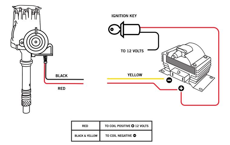
**WARNING:** This distributor is not compatible with stock points distributor coil, must use high output coil. Must bypass ballast resistor if applicable.
