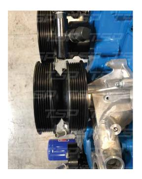
6. This kit requires an additional OEM water pump pulley. Remove the remaining serpentine belt from the driver side of the engine. Remove the bolts holding the water pump pulley in place. The first pulley will be mounted normally. The additional pulley will be mounted reverse. Use supplied M8  $\times$  1.25  $\times$  25mm socket head cap bolts. NOTE: Pulleys are 3 bolt or 4 bolt.
