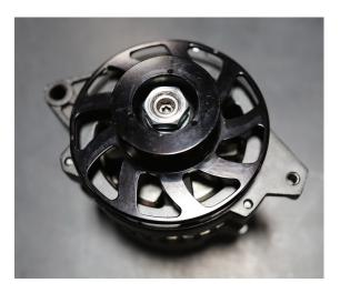
• Using the M4 socket head cap bolts (3), secure the pulley cover to the face of the alternator pulley.
