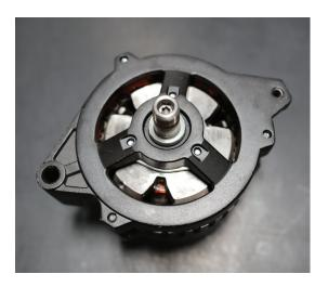
• Once the fan and pulley are removed, install the billet alternator pulley included in the kit. Reinstall the securing nut. Securely tighten to 45 ft/lbs.
