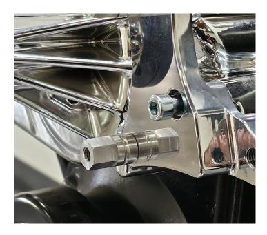
• Install the rear A/C compressor bracket onto the two ears of the water pump on the passenger side. Use supplied M10  $\times$  1.5  $\times$  20mm (2) socket head cap bolts. Securely tighten to 35 ft/lbs.
